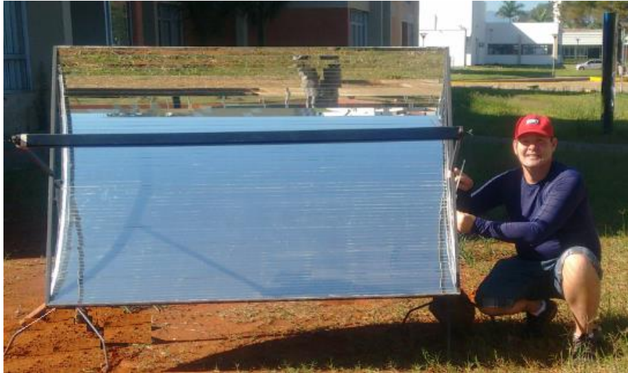
Figura 17 – Solar concentrator in test phase
